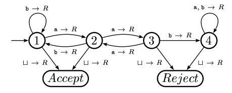
Implicit Reject Convention: To simplify TM state transition diagrams, it is standard to remove the reject state and all arrows (and states) on paths that only lead to the reject state, with the understanding that any transition not accounted for in the diagram implicitly leads to the reject state. Using this convention, our TM can be simplified as follows:
