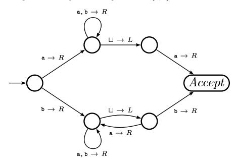
Accepts: any string of the form  $a\Sigma^*a \cup b\Sigma^*b \cup \Sigma$
