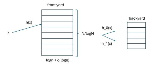
Use single hashing for the front yard, put overflow of frontyard to the backyard using 2 choice hashing.
