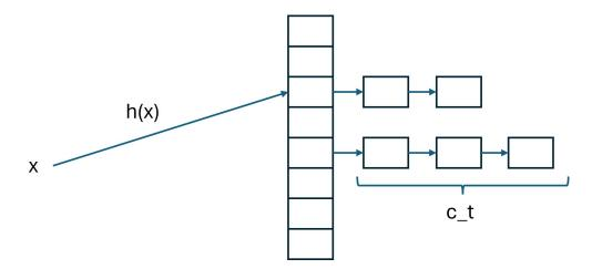
To construct a hash table using perfect hashing, we use the 2-level hashing technique. We store each chain  $c_t$  as a hash table of size  $\theta(c_t^2)$ . After picking a hash function for the first level, we don't want any collisions in the second level of hash tables. We can achieve this by trying hash functions from a universal family of hash functions for the second level. This method only work
