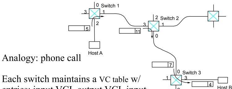
• Each switch maintains a VC table w/ entries: input VCI, output VCI, input port, output port
