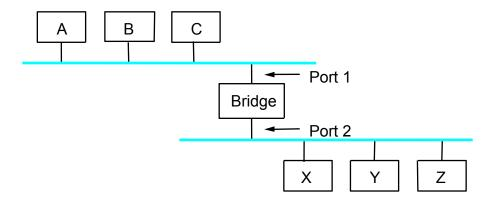
• Ethernet Switch is a LAN Switch = Bridge
