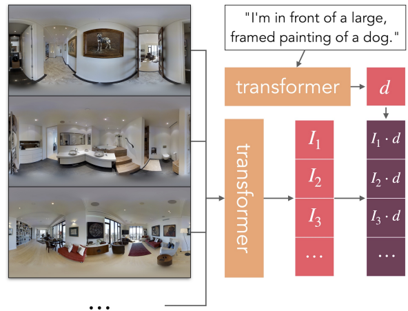
Fig. 4. Model. CLIP [4] uses transformer networks [23], [24] to encode text and images into vectors of identical length, then compares these vectors by taking their dot product. In our task, a description might be compared with as many as 170 images ( views ) from the environment ( scan ).
