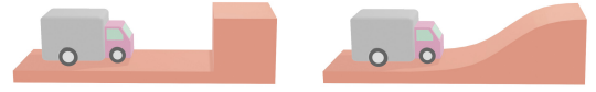
Fig. 5: (left) TDM learns a sharp edge where the velocity is not penalized until at the boundary; (right) the smoothed model penalizes the velocity before reaching the collision boundary.
