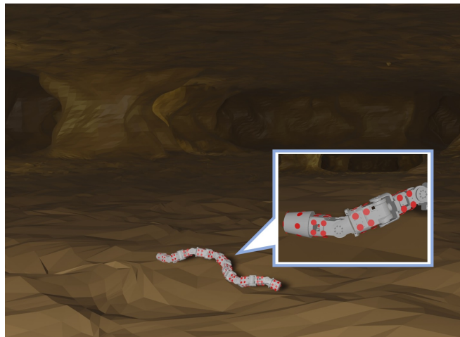
Fig. 1: Snake robot with whole-body tactile sensors performing cave navigation.
