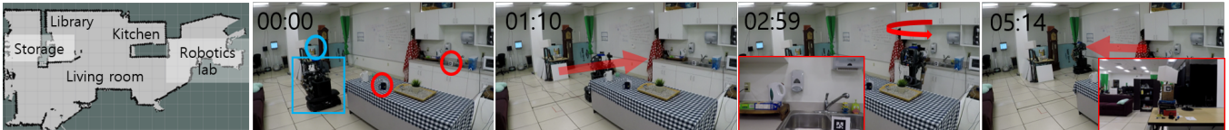
Fig. 4: Experiment with a language command “Find mugs in the kitchen and a book in the library”. The first image shows an occupancy grid map and semantic map of the environment. Red and blue circles indicate mugs and book respectively, and the blue box indicates the robot MOVO. The robot directly moves to the kitchen, looks around, and finds the first mug at 02:59. The inset images (red box) is the robot’s view. The second mug is found in the kitchen at 03:27, after 6 actions. The robot next moves to the library, looks around again, and then finds the book at 05:14 (3 additional actions).
