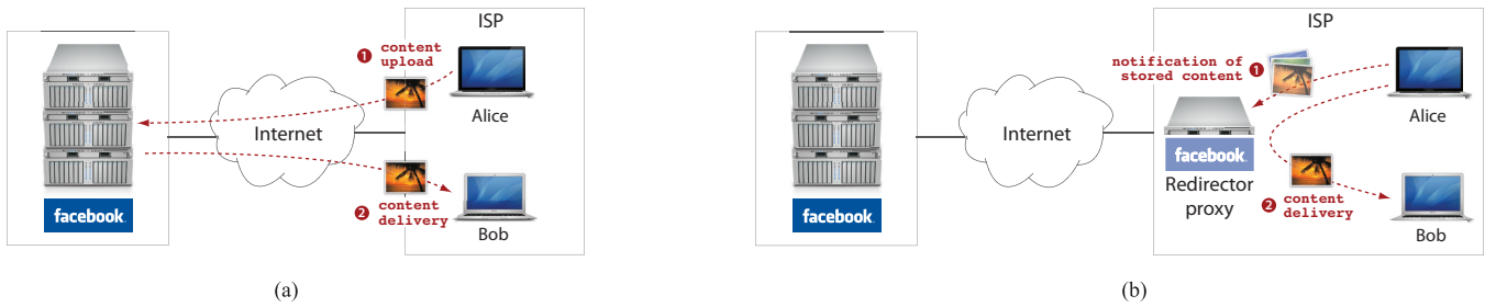
Figure 2. Diagram comparing approaches to content sharing. (a) Content sharing on existing online social networks, where Alice first uploads content to the provider and then Bob requests it. (b) Content sharing in WebCloud, where Alice first informs the proxy of locally stored content. When Bob requests content from the proxy, the proxy fetches it from Alice and delivers it to Bob, thereby keeping the content exchange local.
