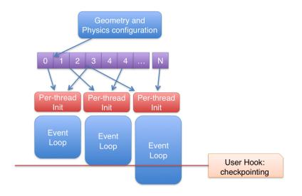
Figure 3. User hook for checkpointing to avoid "tails" CPU cost
