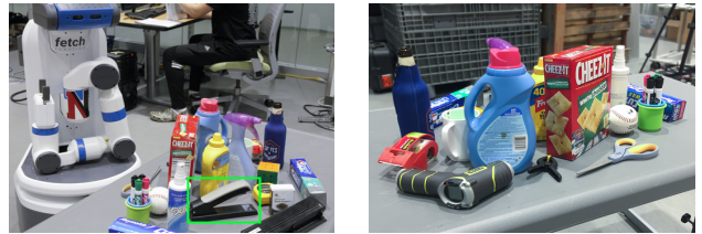
Fig. 1. A service robot is searching for a stapler (Left) which is fully occluded under its current view (Right).
