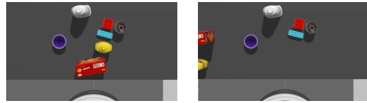
Fig. 7. (Left) Scenario 4 settings (top view). (Right) The challenge of scenario 4 where most of the greedy policies fail by directly grasping the cube without removing tomato can first.
