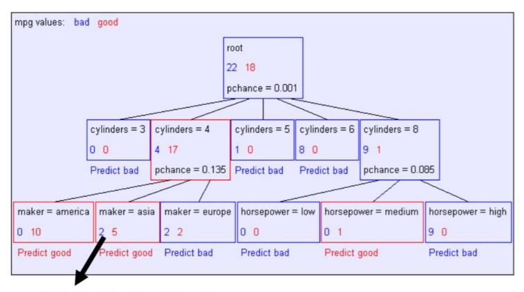
Recursively build a tree from the seven records in which there are four cylinders and the maker was based in Asia
