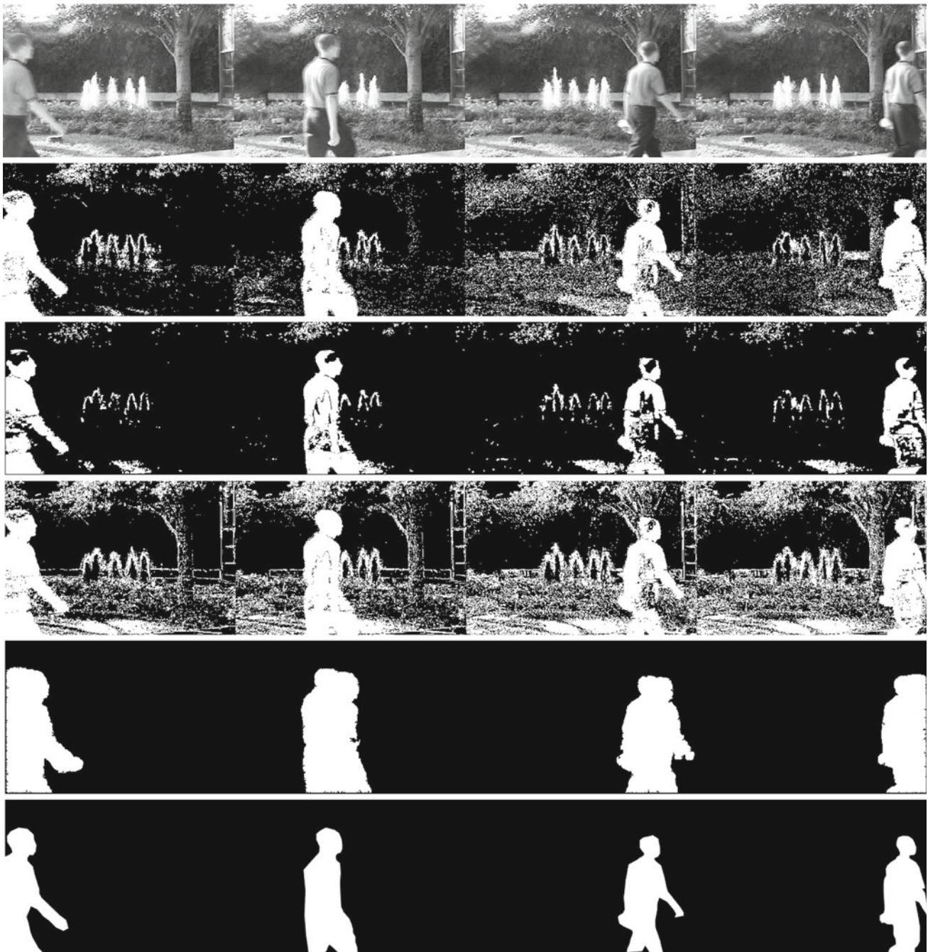
Fig. 2 Experimental results obtained from the fountain sequence. The first row shows the original images followed the results obtained by the mixture of Gaussian approach, shown in row 2 (trained on 400 frames). The results from median-based and principle component analysis-based
