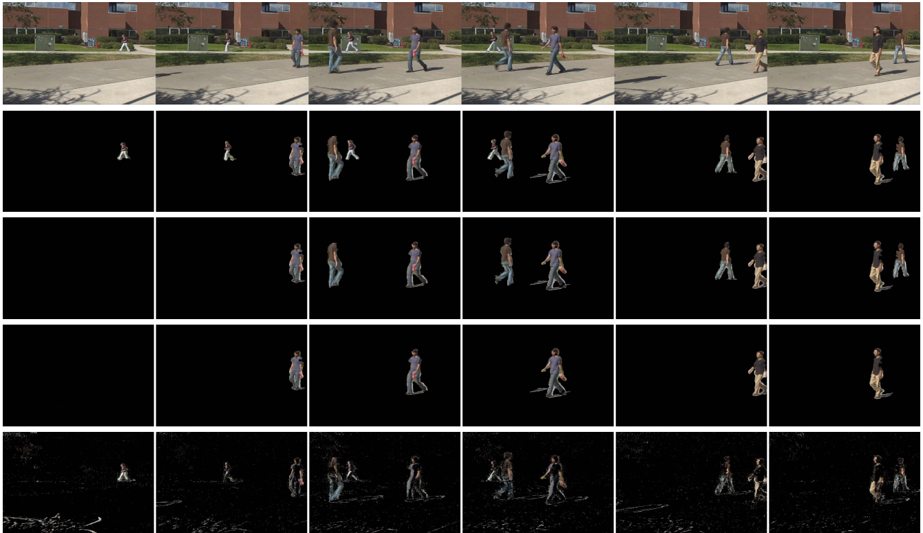
Fig. 1. Selective subtraction results for outdoor sequence: Input images ( first row ), Selective subtraction results with different reference planes ( second to fourth rows ), results from mixture of gaussian method ( last row ).
