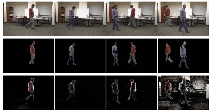
Fig. 3. Selective subtraction results for indoor sequence: Input images ( first row ), Selective subtraction results ( second row ), results from mixture of gaussian method ( last row ).
